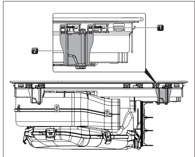
Fig. 6.27 Inserting the cooktop
