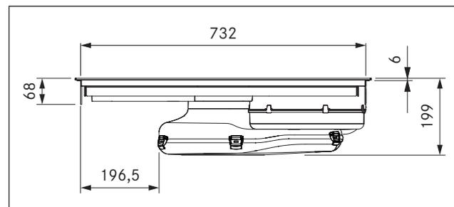
Fig. 3.2 PURA device dimensions front view
