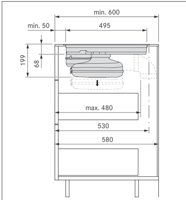
Fig. 6.26 Installation dimensions for exhaust air, worktop depth 600 mm
