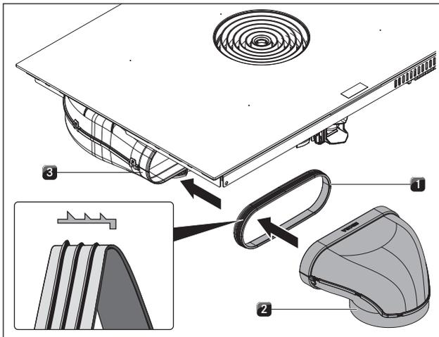
Fig. 6.32 Connecting the duct system
