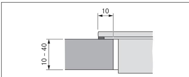
Fig. 6.7 Overlay dimensions for surface mounting
