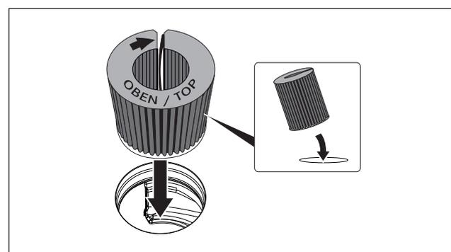
Fig. 6.21 Inserting the activated charcoal filter through the vent opening
