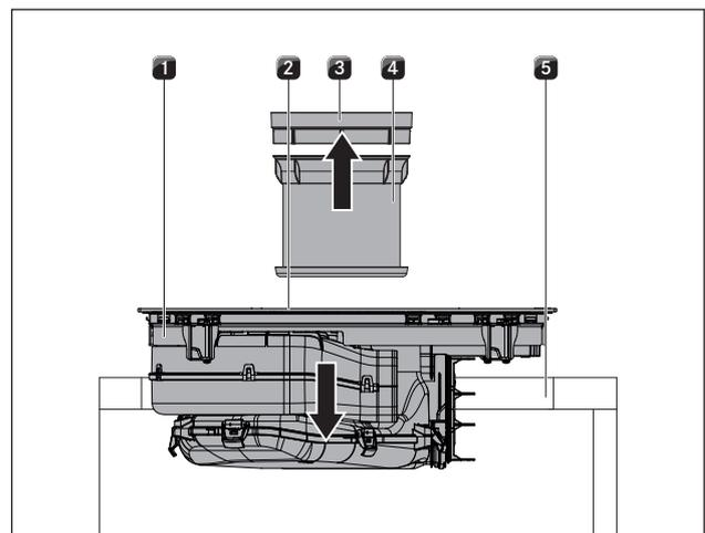
Fig. 6.28 Inserting the cooktop
