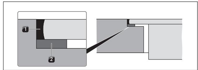
Fig. 6.9 Sealing tape in flush installation
