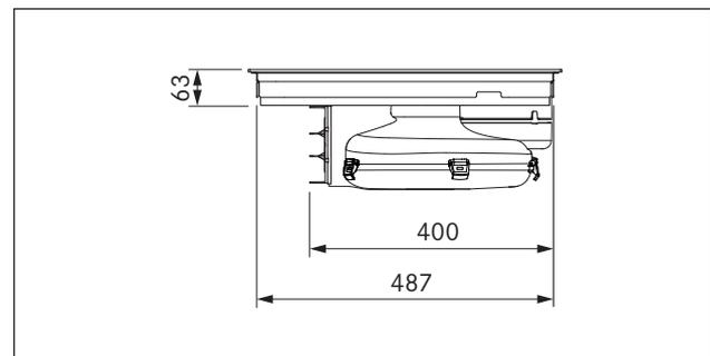
Fig. 3.3 PURA device dimensions side view
