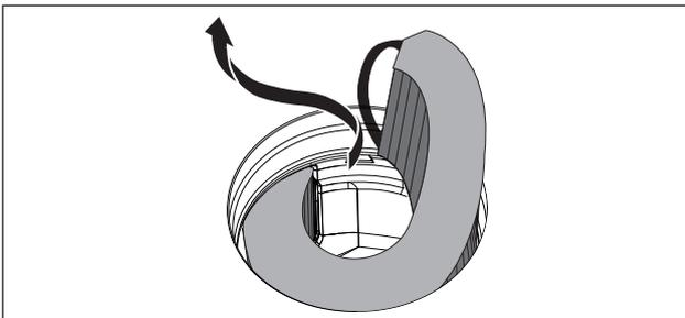
Fig. 8.6 Removing the activated charcoal filter through the inlet opening
