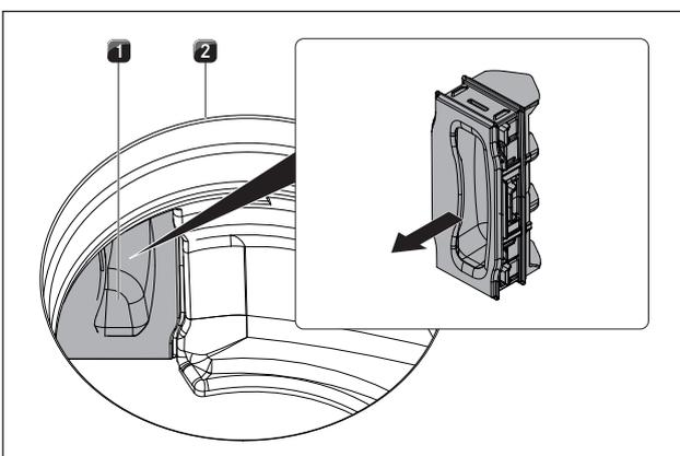
Fig. 6.19 Remove the filter replacement cover
