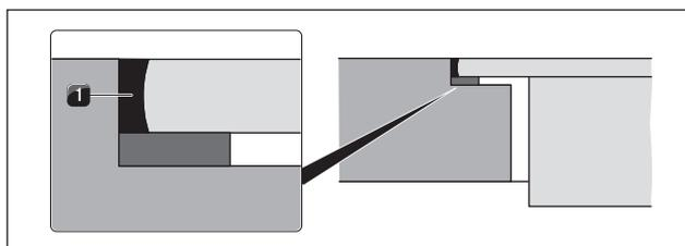
Fig. 6.41 Silicone sealant in flush installation
