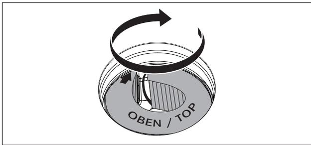
Fig. 6.22 Placing the activated charcoal filter in the end position
