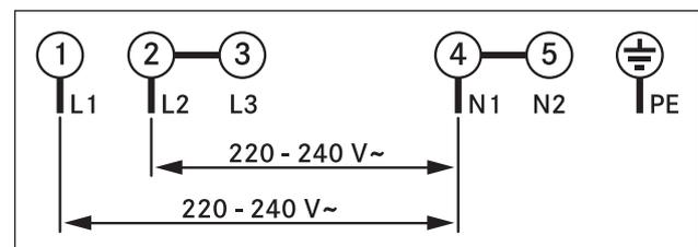
Fig. 6.34 Connection diagram 2-phase connection
