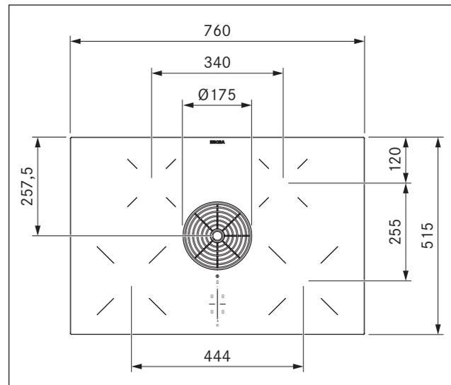
Fig. 3.1 PURA device dimensions top view
