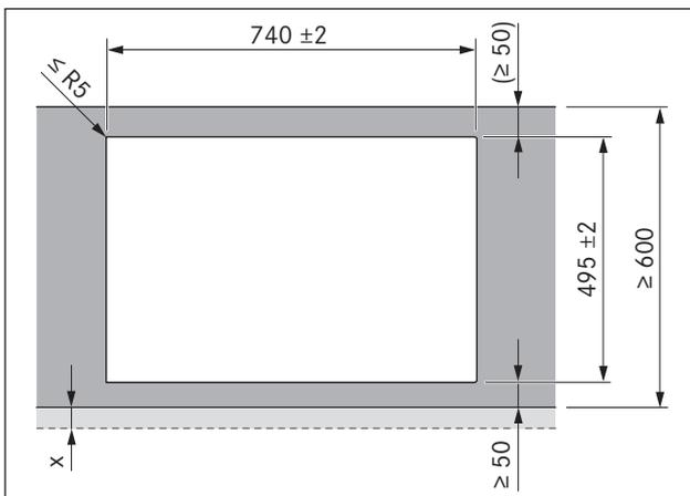
Fig. 6.6 Cut-out dimensions for surface mounting
