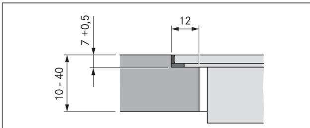
Fig. 6.5 Rebate dimensions for flush installation
