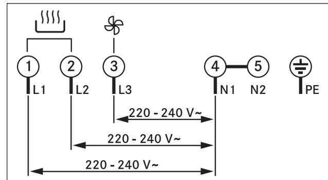
Fig. 6.33 Connection diagram 3-phase connection
