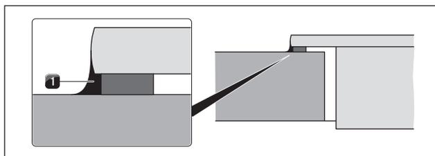
Fig. 6.42 Silicone sealant in surface mounting
