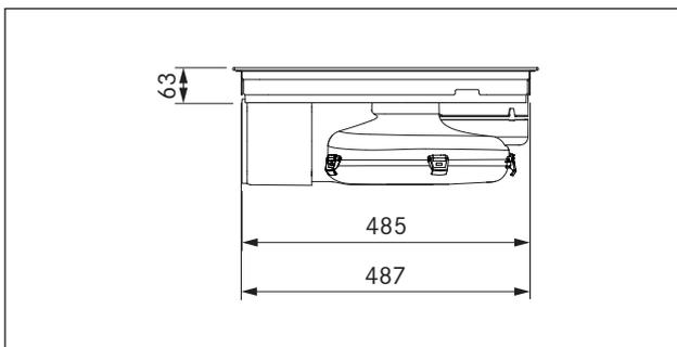
Fig. 3.6 PURA device dimensions side view
