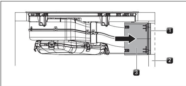
Fig. 6.18 Connecting the telescopic duct to the back wall
