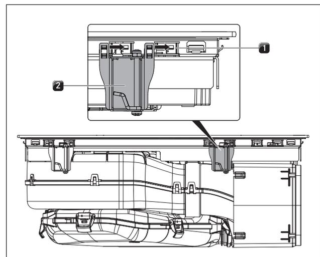
Fig. 6.13 Inserting the cooktop
