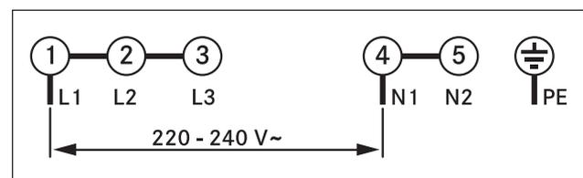
Fig. 6.35 Connection diagram 1-phase connection
